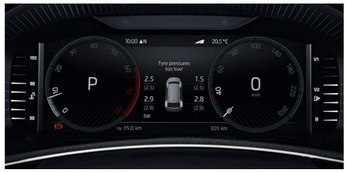
If your vehicle is equipped with optional TPMS (tyre pressure monitoring system with electronic valves) you need to use winter complete wheels with TPMS valves.
